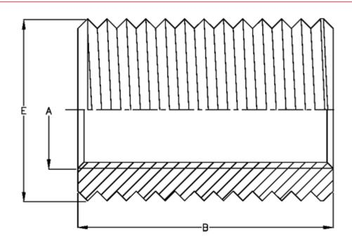
Female thread A = M4Length B = 6 Male thread E = M6 Type = 97x 000 040.120
